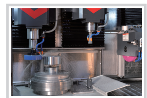
立式主軸 X 2(ID/OD) 臥式主軸 X 1 Vertical spindle x 2(ID/OD) Horizontal spindle x 1
