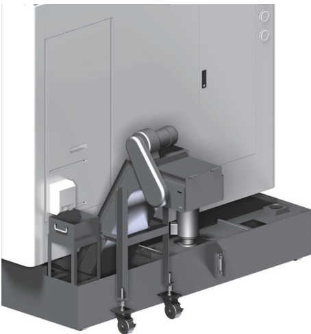
Coolant tank capacity 400 L (80% full)
