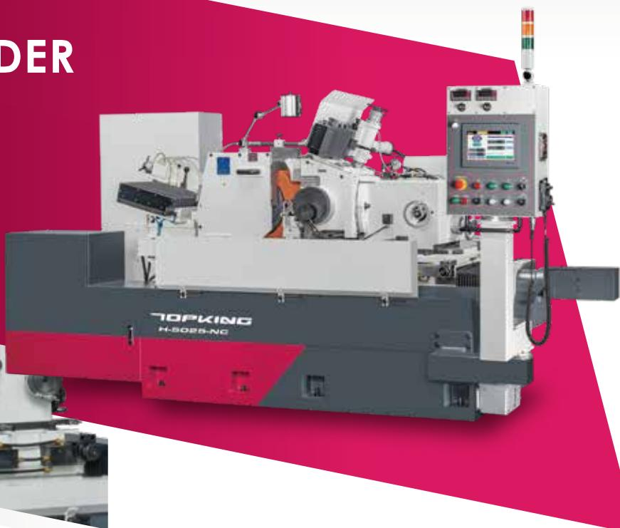
The H Series is built around static pressure technology, offering high precision, low wear, and long-term stability to ensure consistent processing quality. The wheel spindle, regulating wheel spindle, and feeding axis (lower slide rail) are supported by a static pressure oil film, allowing for contact-free operation. This prevents mechanical wear and maintains high precision even during extended use.
