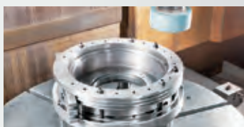
Finishing grinding for brake drum face+ID+OD
