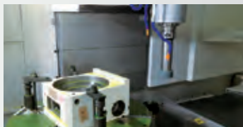
Finishing grinding for casting ID
