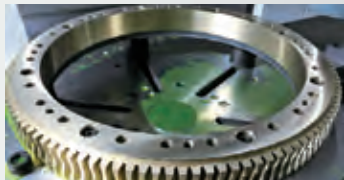
Finishing grinding for gear face
