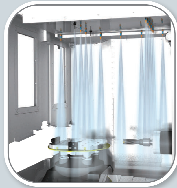
14 Nozzles Coolant Shower
