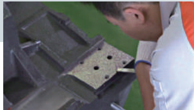
100% Hand-Scraping for Geometry Accuracy and Rigidity
