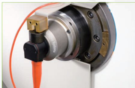
(5) Automatic grinding wheel balancing system Marposs/BS
