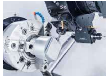
BOTH MAIN AND SUB-SPINDLE HAVE C-AXIS FUNCTION
