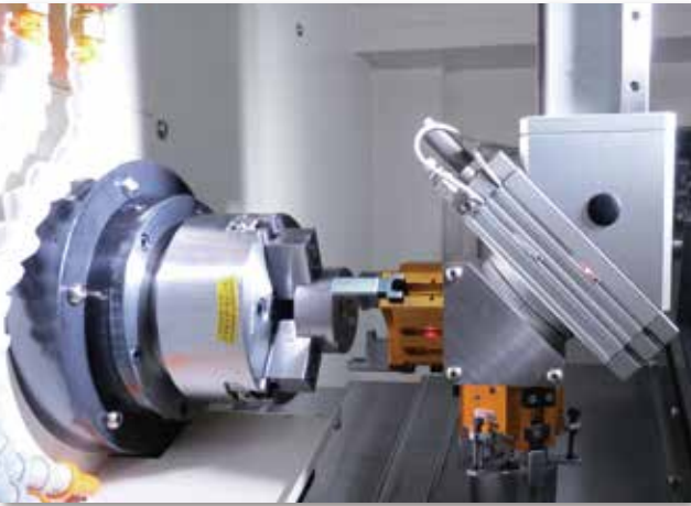
迴轉氣缸含三指定心機械夾爪 Pneumatic rotary air-cylinder with 3-jaw concentric gripper
