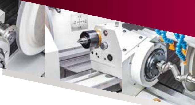
TOPKING's X-CAM series is the specialized design for eccentric and not circular components grinding. It's applied to eccentric, cam shaft, crank shaft, polygon punch grinding. It's especially suitable for use in the automotive, automation equipment, mold industries. Control system equips with advanced SIEMENS controller and cooperates with TOPKING latest GUI work interface, increase parameter setting efficiency. Providing the best accuracy performance and operating environment.
