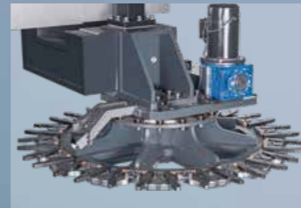
12 Position Armless Type Tool Disk
