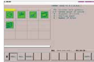
RECTANGULAR HOLE PATTERN (G120 P4) Function
