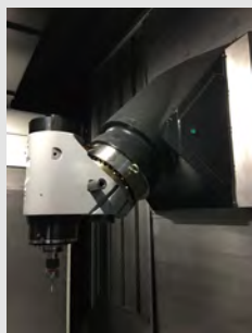
Auto Workpiece Coordinate Measurement & Spindle Clamping / Unclamping Switch
