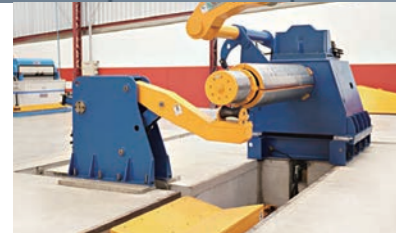
1 Entry Coil Car / Supporting Arm / Uncoiler 上卷台車/支撐臂/開卷機
