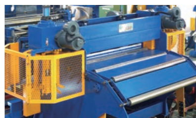
9 Coil End Holder & Scrap Rewinder 尾料壓料及廢料卷取機
