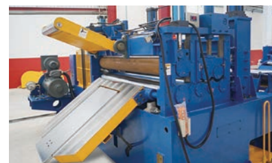
2 Threading & Straightener 入料機構+矯正機
