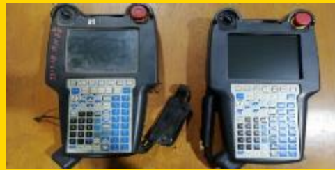
Repair of Teaching Pendant
