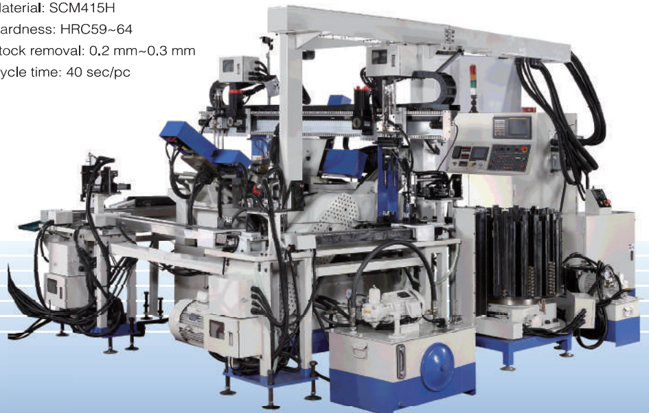
JHC-18 CNC 8 axes with robot system and relay transplanter for grinding universal joint kits. (Rotor system is for loading & unloading)
