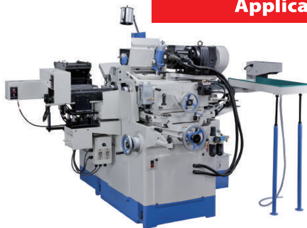
JHC-12S with small size bar feeder & receiver
