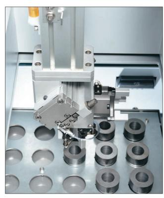
Raw materials or finished products are placed on the tray by robots. Custom trays and stacking requirements can be made for space saving and max storage of up to 12 trays.
