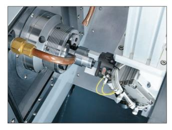
The robot can perform automatic loading and unloading reducing operator input.
