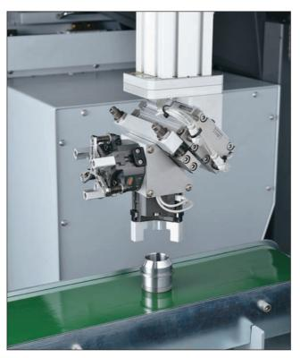
Machine can be equipped with a conveyor
