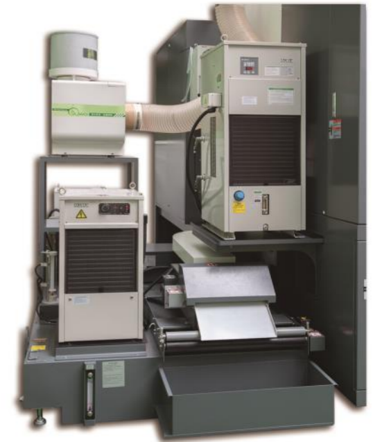
油霧回收器及油冷卻系統 Oil mist collector and cooling system
