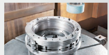
煞車環端面+內外徑研磨
