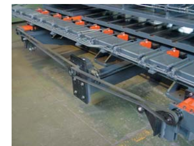
後拖料AC伺服馬達傳動結構 Back sheet support AC servo motor driven structure
