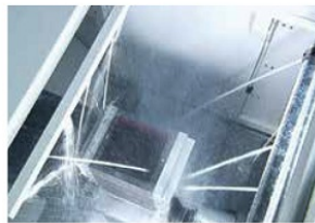
Chip Flushing From Top
