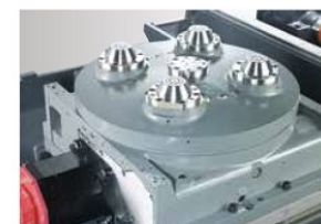
Air Blown from Tapered Cones When pallets are changed to clean any chips for ensuring accuracy and pallet positioning.
