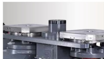
Pallet Changer The pallet is driven by servo motor.
