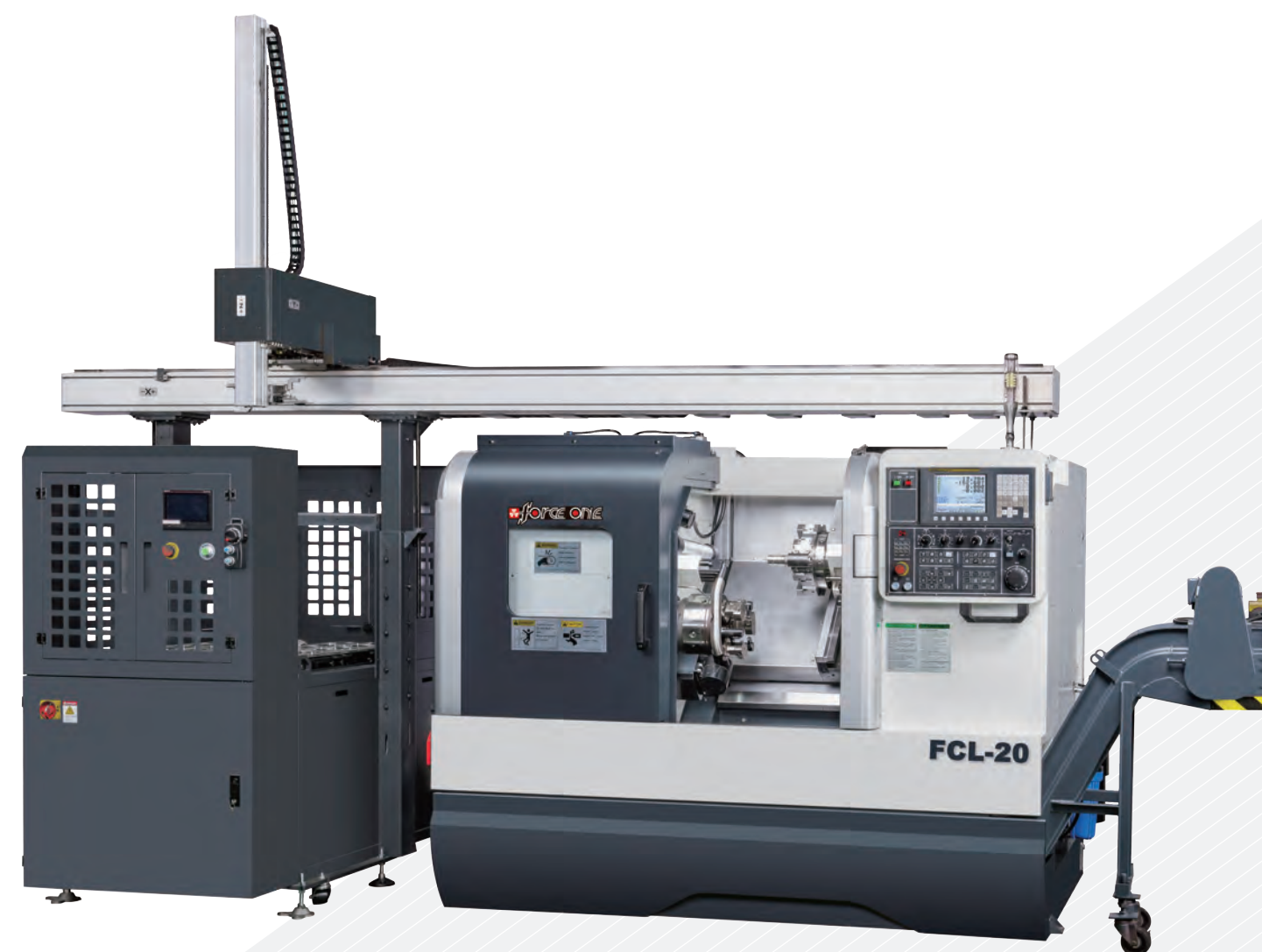
FCL SERIES WITH GANTRY LOADING SYSTEM (OPT.)
