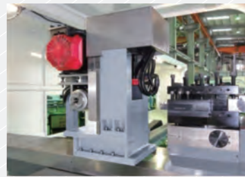
Driving tool with Y axis + spindle with CS / CF (option) is available.
