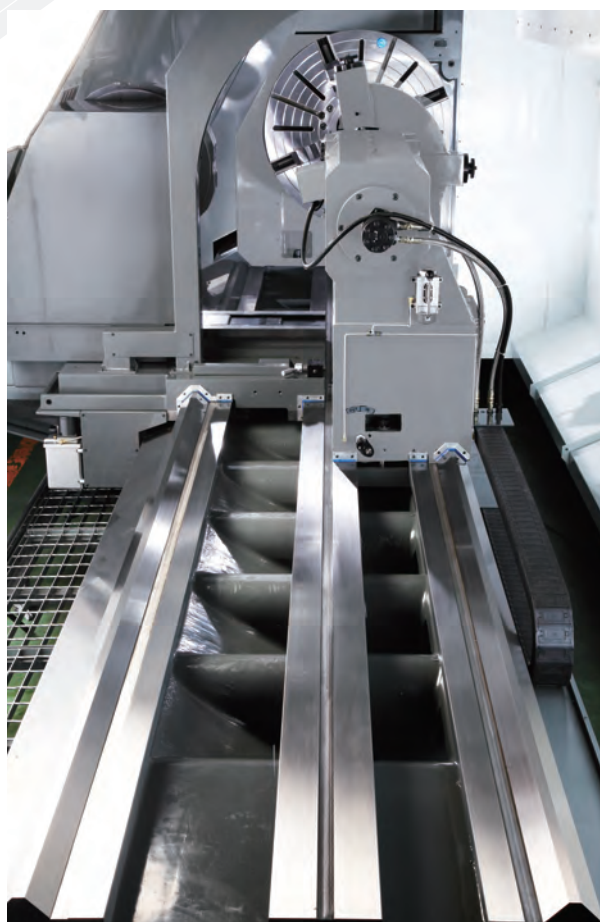
4 Bed Ways With Half Length Saddle
